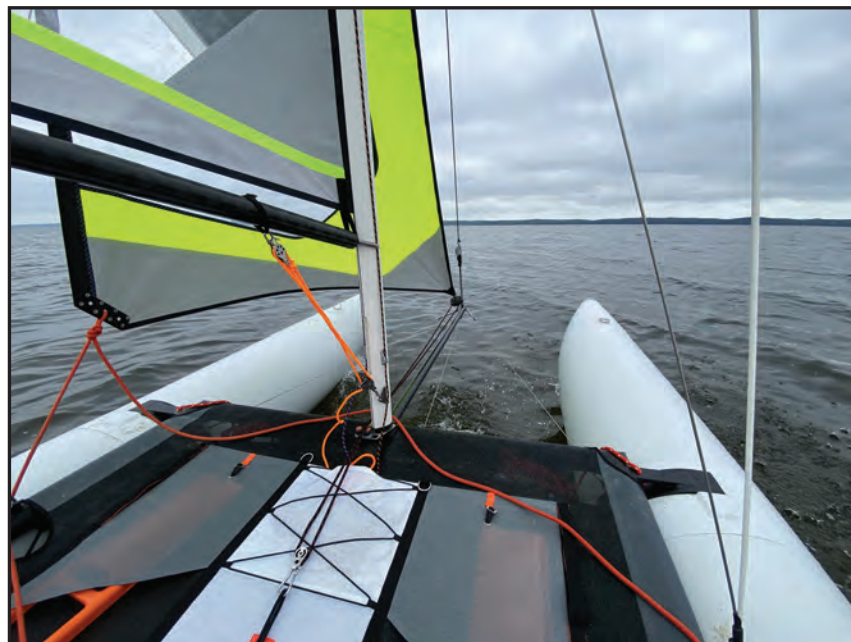
Sitting on the trampoline and the tubes is very comfortable. The off-center sheeting points for the genoa mean you can't sail tightly close-hauled.
