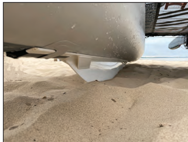
The skegs - especially the reinforcing sections - could do with hydrodynamic optimization.
