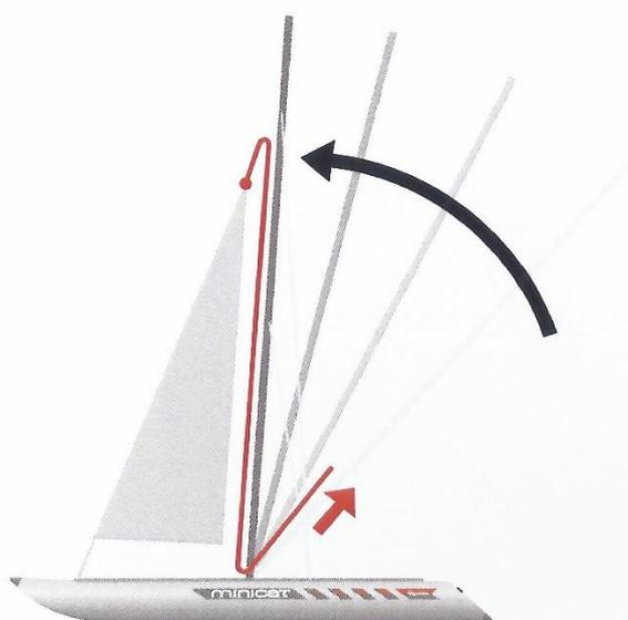
The mast is now raised and the jib is stretched. Roll up the jib using the furler rope loop so that it does not flap in the wind. Attach the furler rope loop to the eye on the mast with a carabiner. Attach the end of the rope with the pulley to the sheet metal under the mast joint. Thread the jib sheet reins through the clamps on the side parts of the frame.
