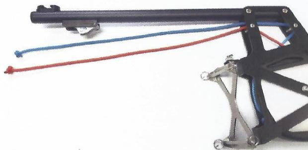
**Rudder lever with lines**
